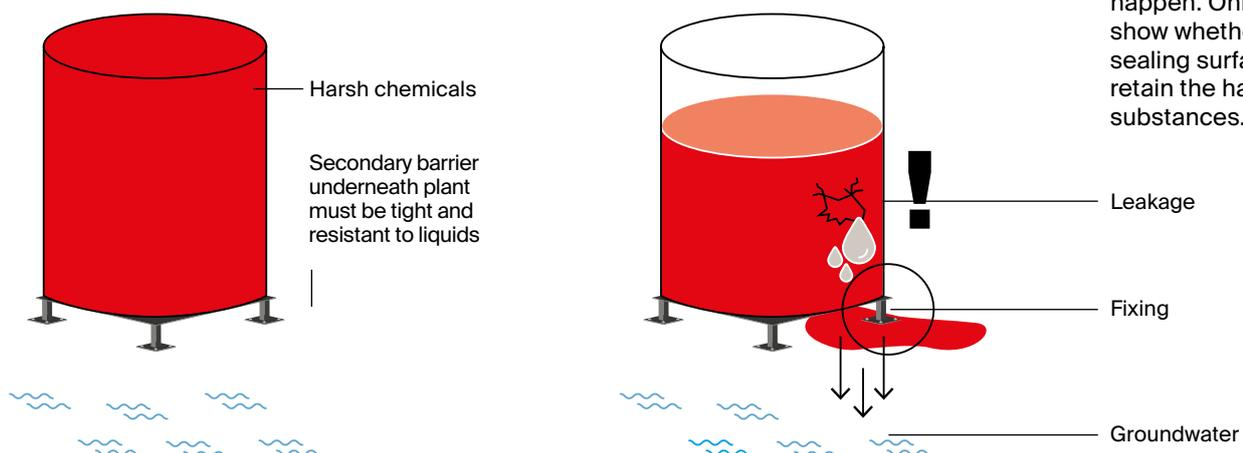
Accidents can always happen. Only then will it show whether the sealing surface can fully retain the hazardous substances.
