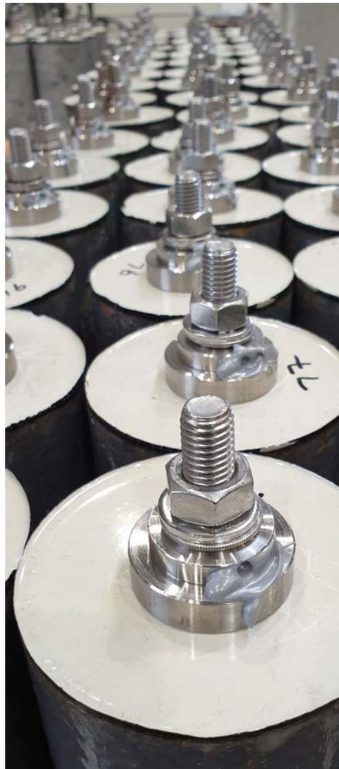
Anchoring systems have to be tested in elaborate test series. Here you can see test cylinders being sampled from a coated concrete surface.
