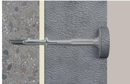
Countersunk installation of polystyrene boards on concrete
