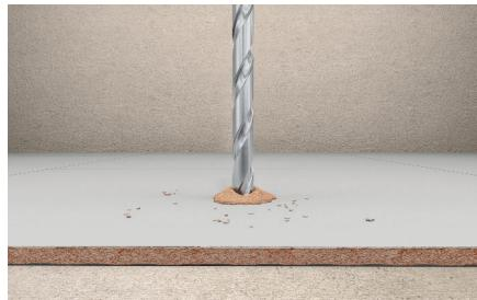
Drilling the material combination tile and concrete
