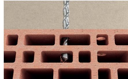
Cross section of hollow brick drilling
