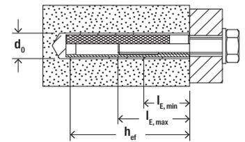
Internal threaded anchor FIS E: Application in solid masonry, perforated brick masonry and aerated concrete
