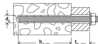
Threaded rod FIS A: Application in concrete
