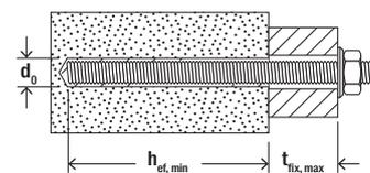
Threaded rod FIS A: Application in solid masonry, perforated brick masonry and aerated concrete
