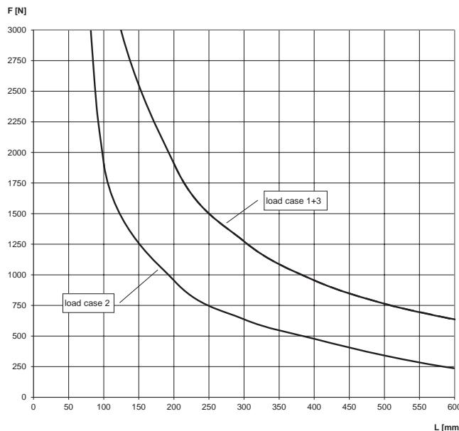
For the load curves, the permissible steel strain  $\delta_{\text{adm.}} = 188 \text{ N/mm}^2$  (increased steel strain due to bending) and the maximum deflection under load  $L/150$  are not exceeded. Fixings and screw fastenings must be calculated accordingly.
