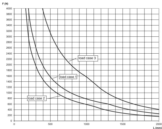
For the load curves, the permissible steel strain  $\delta_{\text{adm.}} = 188 \text{ N/mm}$  (increased steel strain due to bending) and the maximum deflection under load  $L/200$  are not exceeded. Fixings and screw fastenings must be calculated accordingly. The higher yield strength is a result of the calculation according to DIN EN 1993-1-3:2010-12, para. 3.2.2.
