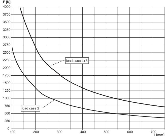
For the load curves, the permissible steel strain  $\delta_{\text{adm.}} = 160 \text{ N/mm}$  and the maximum deflection under load  $L/150$  are not exceeded. Load values of the cantilever arms under consideration of the load capacity of the base plate. Fixings and screw fastenings must be calculated accordingly.
