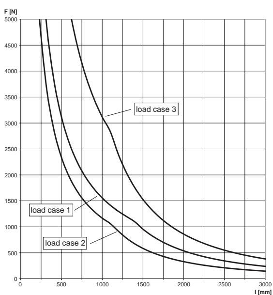
For the load curves, the permissible steel strain  $\delta_{\text{adm.}} = 188 \text{ N/mm}$  and the maximum deflection under load  $L/200$  are not exceeded. Fixings and screw fastenings must be calculated accordingly. The increased yield strength is calculated according DIN EN 1993-1-3:2010-12, sec. 3.2.2.
