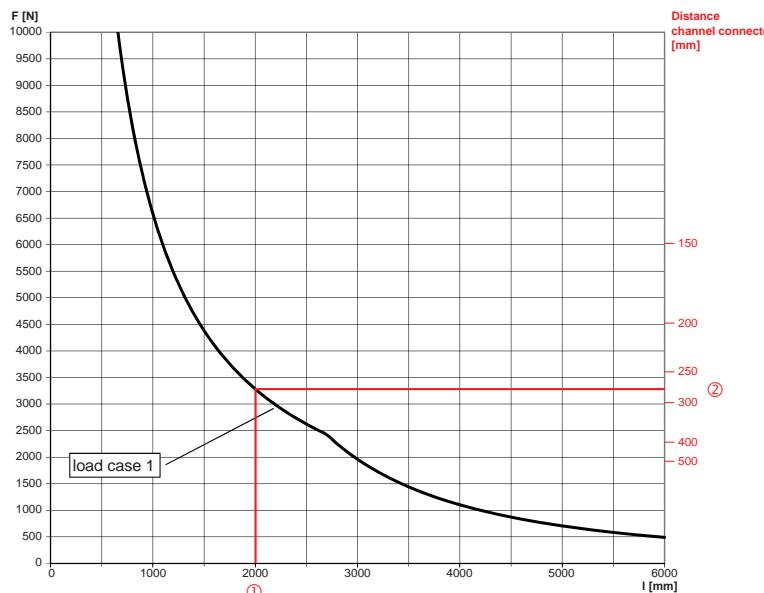
① Length of channel, i.e. 2000 mm for loadcase 1 (single load centric)
