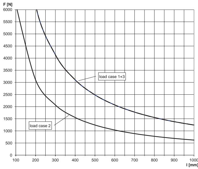
For the load curves, the permissible steel strain  $\delta_{\text{adm.}} = 160 \text{ N/mm}$  and the maximum deflection under load  $L/150$  are not exceeded. Load values of the cantilever arms under consideration of the load capacity of the base plate. Fixings and screw fastenings must be calculated accordingly.
