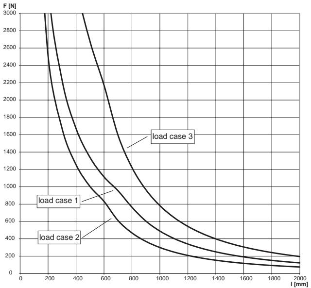
For the load curves, the permissible steel strain  $\delta_{\text{adm.}} = 188 \text{ N/mm}$  and the maximum deflection under load  $L/200$  are not exceeded. Fixings and screw fastenings must be calculated accordingly. The increased yield strength is calculated according DIN EN 1993-1-3:2010-12, sec. 3.2.2.
