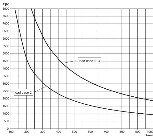
For the load curves, the permissible steel strain  $\delta_{\text{adm.}} = 160 \text{ N/mm}$  and the maximum deflection under load  $L/150$  are not exceeded. Load capacity for console under consideration of the capacity of base plate. Fixings and screw fastenings must be calculated accordingly.
