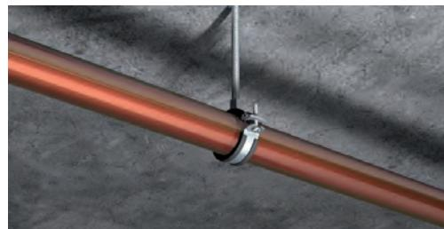
In most cases, pipes and supply lines are installed in dry rooms. Therefore, in addition to corrosion resistant materials, such as plastics or stainless steel and copper, the steel products used for installation systems are galvanised. A zinc coating thickness of 5-8 µm by means of electrolytic process (galvanising) is standard.
