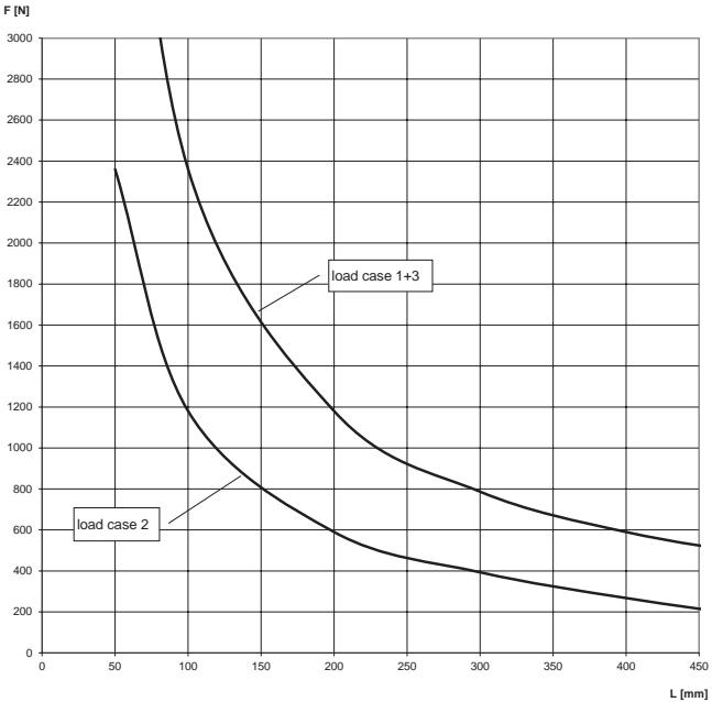
For the load curves, the permissible steel strain  $\delta_{adm.} = 188 \text{ N/mm}^2$  (increased steel strain due to bending) and the maximum deflection under load L/150 are not exceeded. Fixings and screw fastenings must be calculated accordingly.
