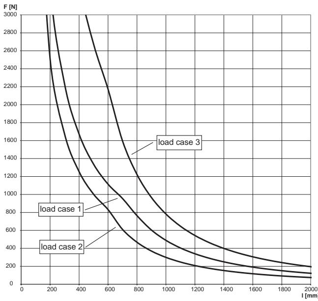
For the load curves, the permissible steel strain  $\delta_{\text{adm.}} = 188 \text{ N/mm}$  and the maximum deflection under load  $L/200$  are not exceeded. Fixings and screw fastenings must be calculated accordingly. The increased yield strength is calculated according DIN EN 1993-1-3:2010-12, sec. 3.2.2.
