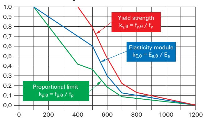
Dependency of the yield strength, proportional limit and elasticity module on the temperature (basis: EN1993-1-2:2012-12 Eurocode 3).
