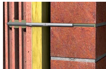
Detail: Repairing outer leaves
