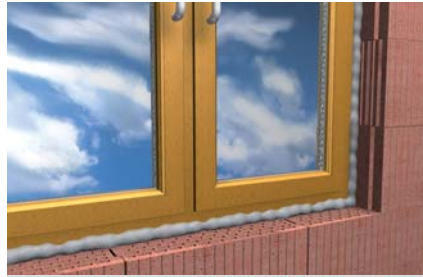
Window connection joints
