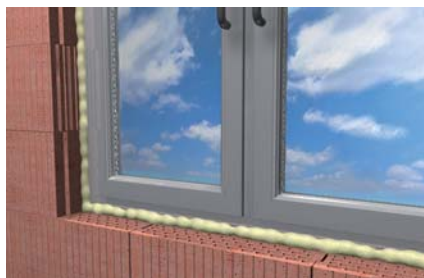
Window connection joints
